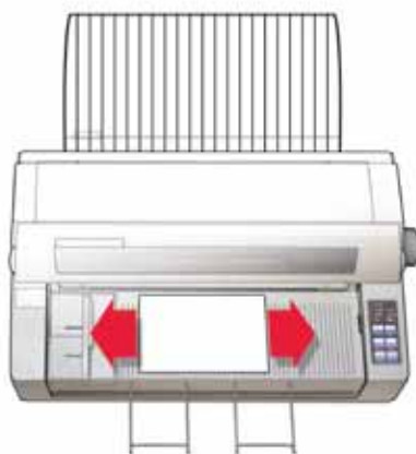
Media can be hand-fed at virtually any point across printer table
